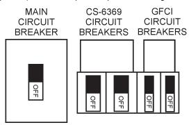
Figure 38. Main, Aux. and GFCI Circuit Breakers (OFF)
